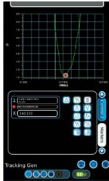
Tracking generator showing VSWR graph
