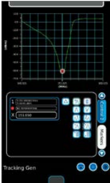
Tracking generator tuning a duplexer
